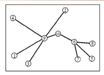
Fig. 2: Broadcast tree using BIP
