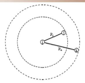
Fig. 1: The "wireless multicast advantage":  $P_{t,(j,k)} = \max\{P_{ij}, P_{ik}\}$
