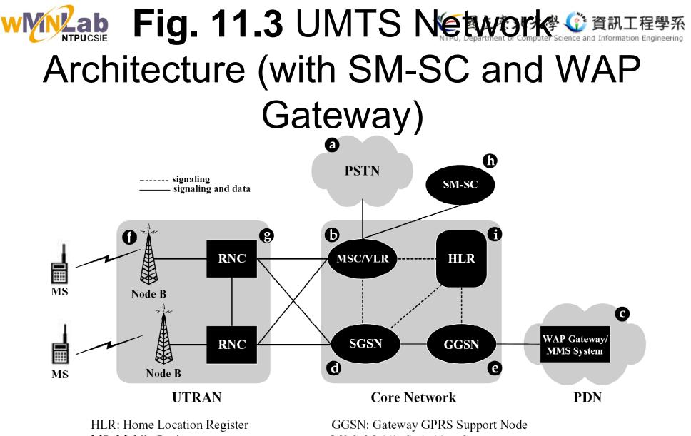
MS: Mobile Station PSTN: Public Switched Telephone Network SGSN: Serving GPRS Support Node VLR: Visitor Location Register PDN: Packet Data Network GGSN: Gateway GPRS Support Node MSC: Mobile Switching Center RNC: Radio Network Controller SM-SC: Short Message Service Center Node B: Base Station UTRAN: UMTS Terrestrial Radio Access Network
