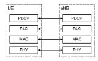
**PDCP** is an abbreviation for Packet Data Convergence Protocol. It is one of the layers of the Radio Traffic Stack in <u>UMTS</u> and performs <u>IP</u> header compression and decompression, transfer of user data and maintenance of sequence numbers for Radio Bearers which are configured for <u>lossless</u> serving radio network subsystem (SRNS) relocation.
