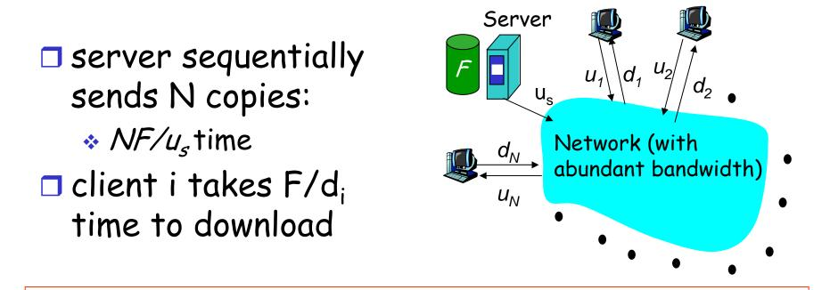
Time to distribute Fto N clients using =  $d_{cs} = max \{ NF/u_{s}, F/min(d_i) \}$ client/server approach
