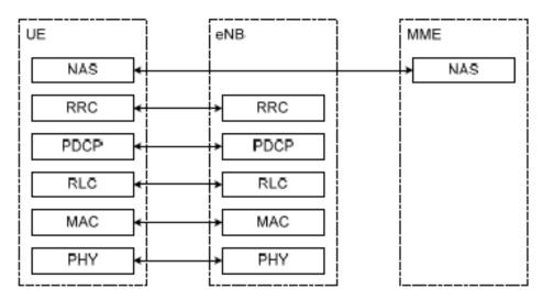
Non Access Stratum (NAS) is a functional layer in the <u>UMTS</u> <u>protocol stack</u> between Core Network and User Equipment <u>UE</u>. The layer supports signalling and traffic between those two elements.
