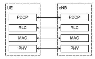
**PDCP** is an abbreviation for Packet Data Convergence Protocol. It is one of the layers of the Radio Traffic Stack in <u>UMTS</u> and performs <u>IP</u> header compression and decompression, transfer of user data and maintenance of sequence numbers for Radio Bearers which are configured for <u>lossless</u> serving radio network subsystem (SRNS) relocation.
