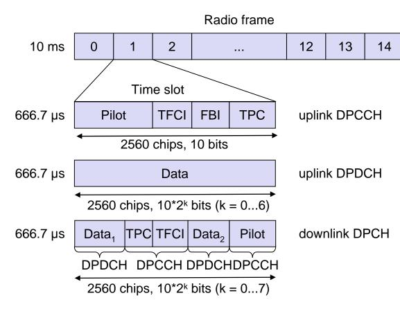
Slot structure NOT for user separation but synchronisation for periodic functions!
