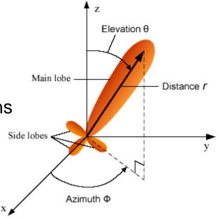
When  $U(\theta, \phi) = U_{ave}$  the antenna is called **isotropic**.
