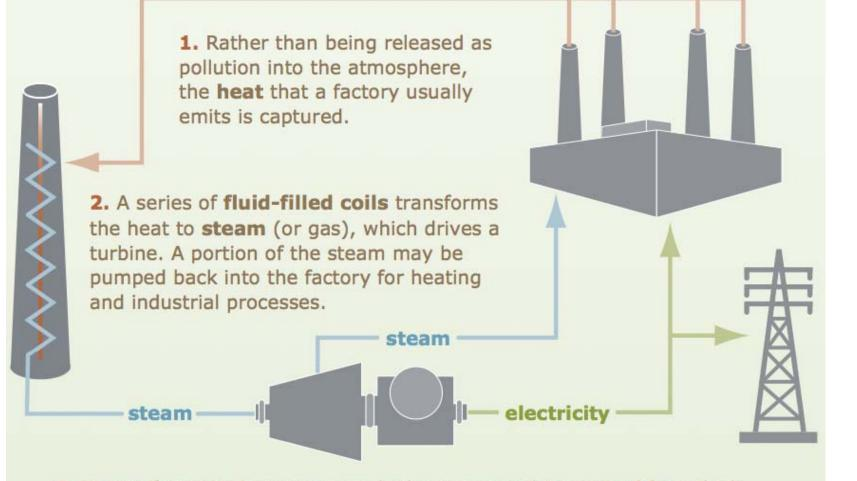
**3.** Steam from the heat recovery boiler is pumped into a **turbine** which generates electricity used to power the plant. Excess power may be sent to the local grid to provide clean electricity for the outlying community.
