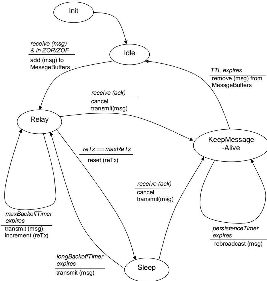
Figure 3.9: Finite state machine for distributed robust geocast
