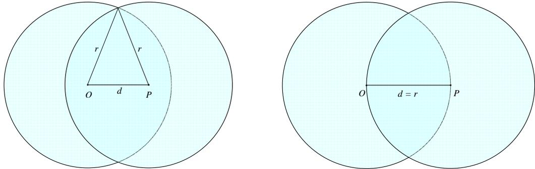
(a) Two nodes at a distance less than transmission range      (b) Two nodes at a distance equal to transmission range
