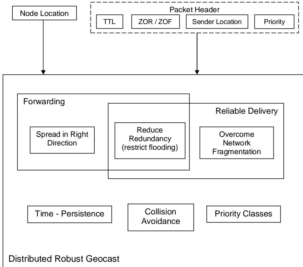
Figure 3.1: Architecture for Distributed Robust Geocast
