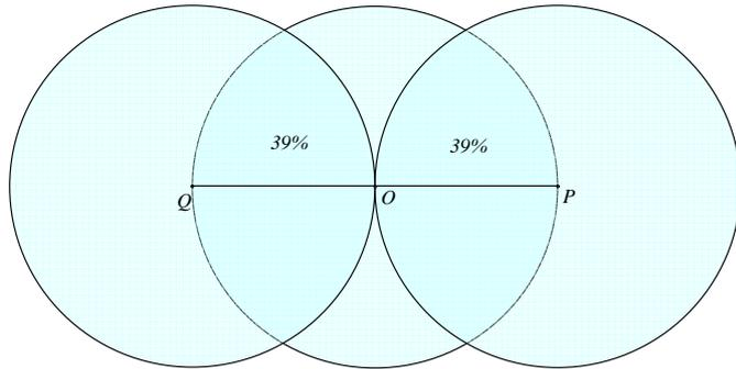
Figure 3.6: Two nodes on the edge of center node's transmission range
