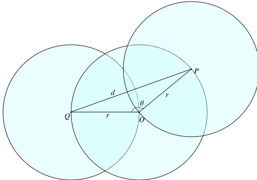
Figure 3.8: Two nodes on the edge of center node's transmission range, forming an angle  $\theta$  at the center node
