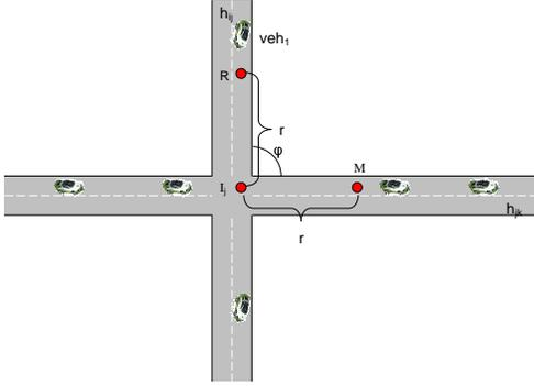
Fig. 1. Representation of an intersection in a road network presenting the basic notations
