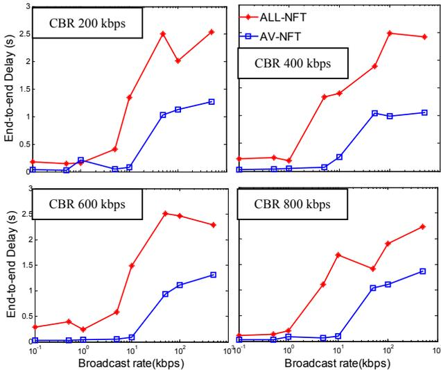
Figure 16. End-to-End delay of ALL-NFT and AV-NFT
