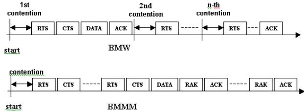
Figure 2. Timing Diagrams of BMW and BMMM
