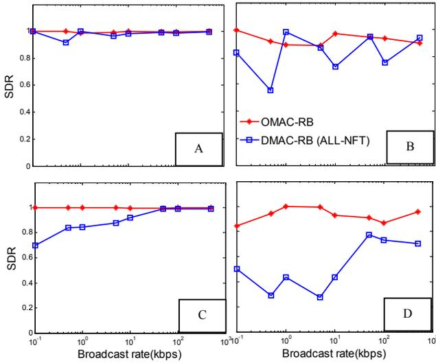
**Figure 11. A & B show SDR at 50% and 80% reliability threshold respectively for CBR 200kbps; C & D show SDR at 50% and 80% reliability threshold respectively for CBR 800kbps**
