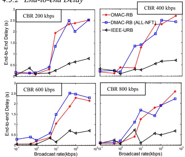
**Figure 10. End-to-end delay for CBR rates 200kbps, 400kbps, 600kbps & 800kbps**
