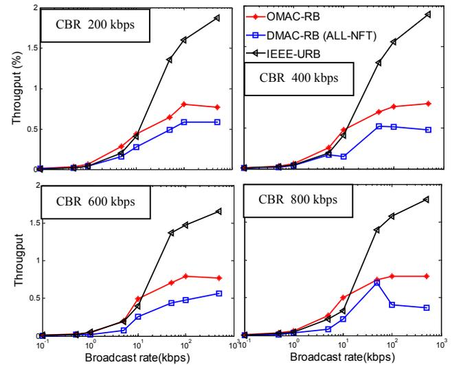
**Figure 6. Throughput for different CBR rates**
