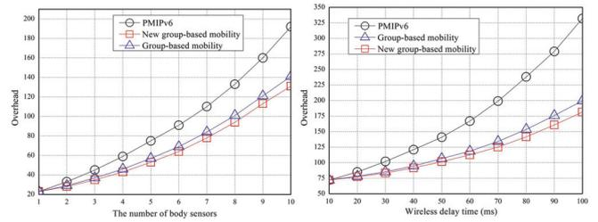
Fig. 14. Performance of overhead vs. (a) The number of sensors. (b) Wireless link delay.
