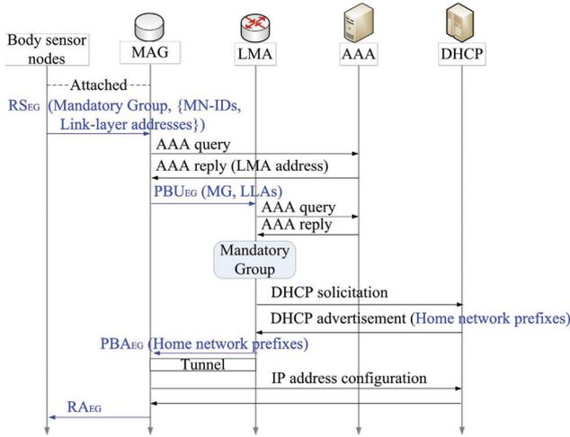
Fig. 7. The signaling call flow for the proposed registration scheme.
