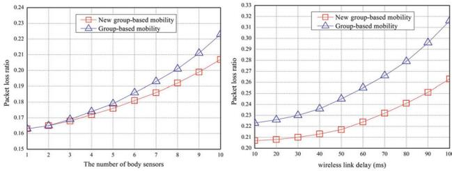
Fig. 12. Performance of packet loss ratio vs. (a) The number of sensors. (b) Wireless link delay.
