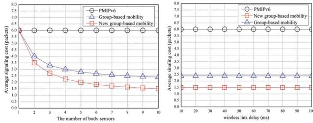
Fig. 13. Performance of average signaling cost vs. (a) The number of sensors. (b) Wireless link delay.
