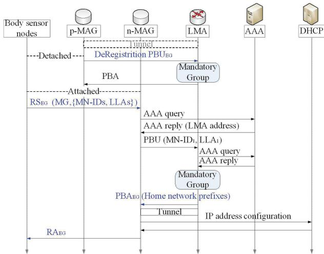
Fig. 9. The signaling call flow for the proposed handoff scheme.
