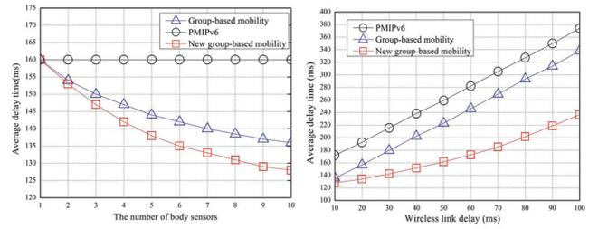
Fig. 11. Performance of average delay time vs. (a) The number of sensors. (b) Wireless link delay.
