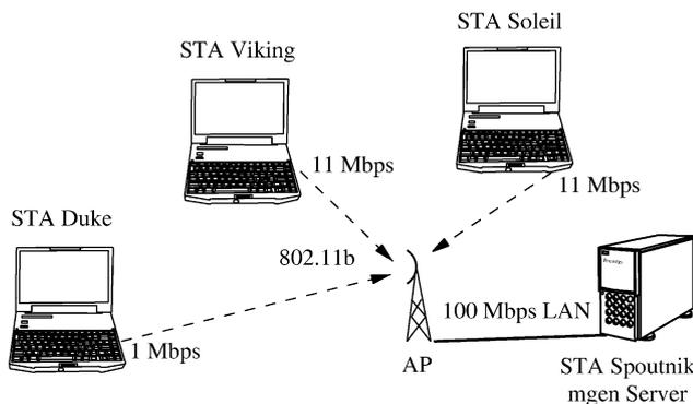
Fig. 3. Experiment setup in our 802.11b testbed.
