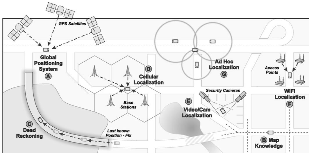
Fig. 3. Examples of localization techniques applied in VANets.
