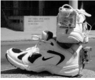
Fig. 11. Functional prototype of piezoelectric-powered RFID shoes with mounted electronics[22].
